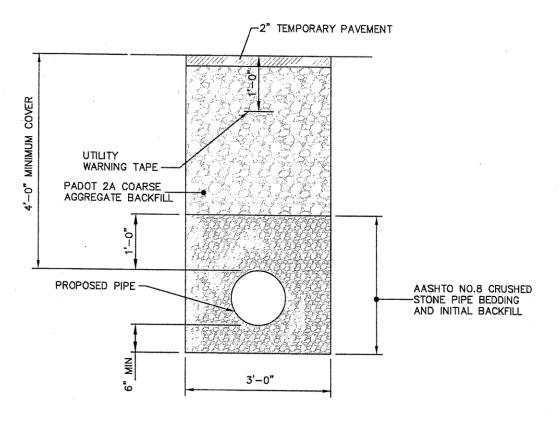
AGGREGATE BACKFILL AND PAVEMENT MATERIALS AND THEIR INSTALLATION SHALL BE IN ACCORDANCE WITH COMMONWEALTH OF PENNSYLVANIA DEPARTMENT OF TRANSPORTATION SPECIFICATION PUBLICATION 408, LATEST EDITION.
